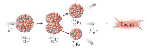
The nuclides produced in the reaction pictured above are only two of many possible fission products of uranium-235. More than 200 different nuclides form, representing 35 different elements. Two possible reactions are
