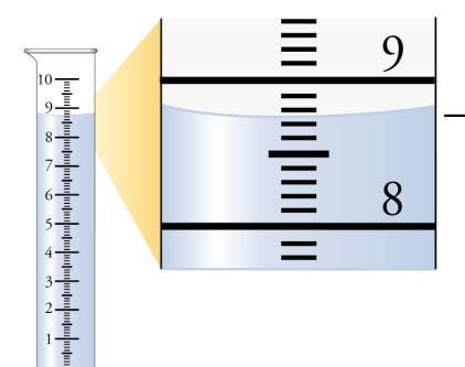
Comparing the position of the bottom of the meniscus and the milliliter scale yields a measurement of 8.74 mL.
